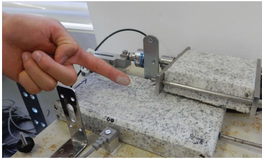
Figure 9. A view of a sheared rough saw-cut discontinuity plane with a thin powder after testing.
