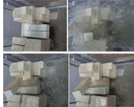
Figure 17. Top views of the plaster block overhanging over the base Ryukyu limestone blocks at different time steps.
