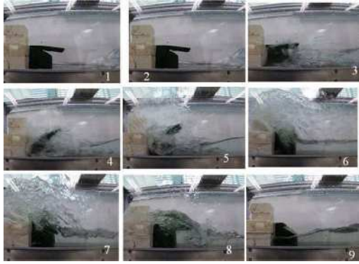
Figure 19. Views of the experiments using a breakable overhanging block at different time steps.
