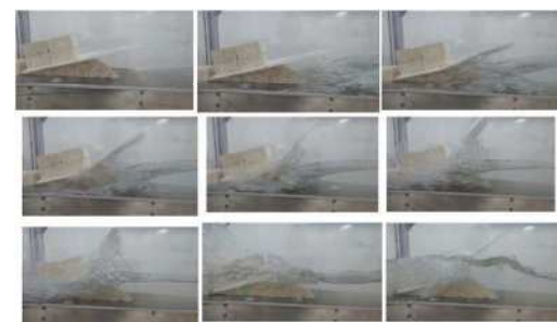
Figure 18. Views of the experiments using a breakable overhanging block at different time steps.
