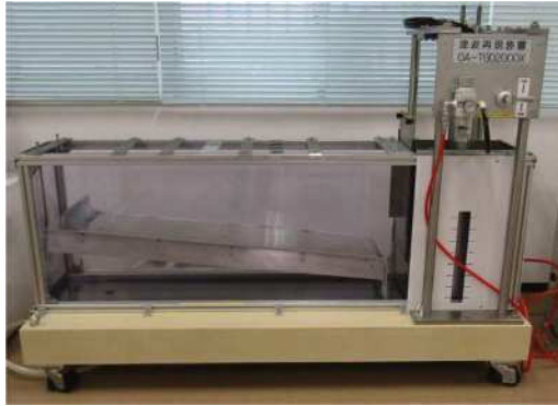
Figure 5. A view of the tsunami generation device OA-TGD2000X.
