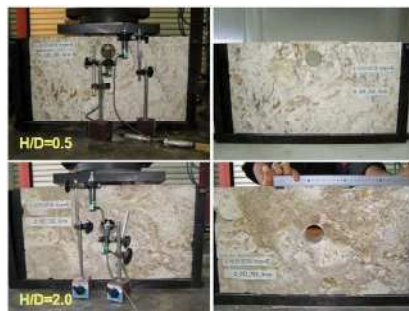
Figure 22. Experiment on the effect caves on footing separation.
