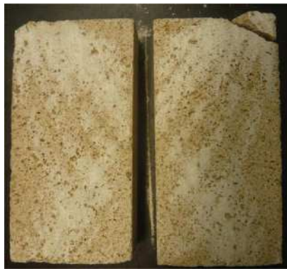
Figure 13. A view of a saw-cut discontinuity plane after a direct shear test.
