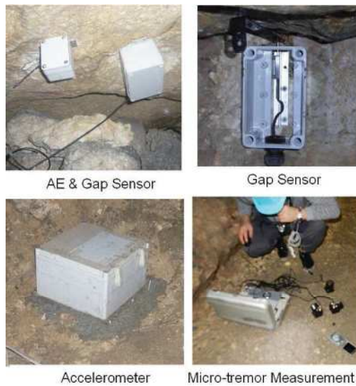
Figure 14. Instrumentation for multi-parameter monitoring
