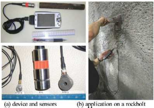
Figure 10. Non-destructive test device and its utilization on a rockbolt in the access tunnel.
