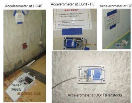
Figure 7. Views of installed accelerometers.
