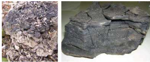
Figure 7. Examples of disintegration of soft rocks of Mitake.
